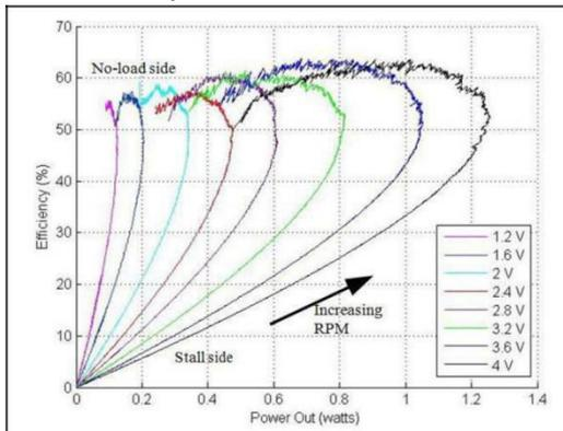
**Fig3.1** Efficiency vs. motor power output for the brushed motor.
